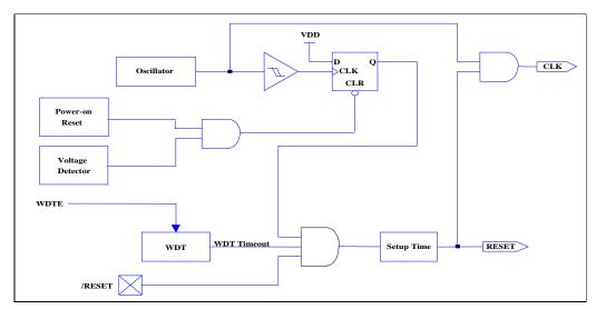
Fig. 5-28 Controller Reset Block Diagram
